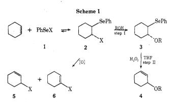
Unlike previous procedures<sup>1</sup> we have found it desirable to isolate<sup>5</sup> the intermediate adducts (3), which were oxidized (H<sub>2</sub>O<sub>2</sub>, THF) in a separate step to the desired unsaturated products. Table I reveals that the overall yields for this two-step procedure are quite good.
